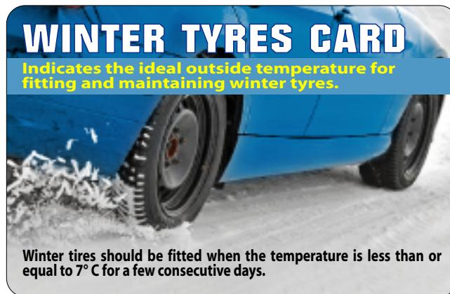
Winter tires should be fitted when the temperature is less than or equal to 7°C for a few consecutive days.
